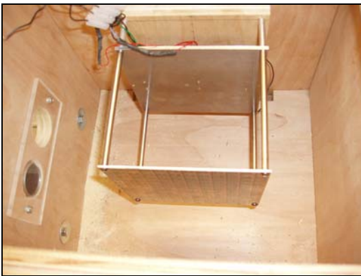
Figure 15: The plate is mounted directly in front of the beamline on an adjustable backing plate. Notice the camera lens at left.
