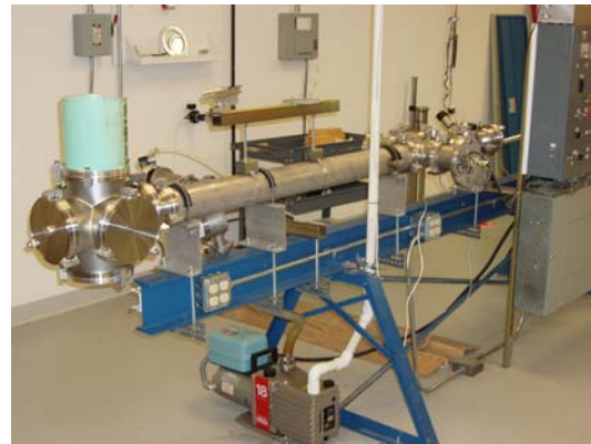
Figure 13: The CASPER LGG uses helium at 500-1000 psi to fire projectiles up to 800 m/s. A laser fan is used to determine the velocity of the projectile. The LGG was run under normal atmospheric pressure rather than under vacuum as in previous experiments.
