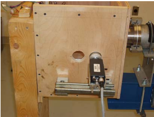
Figure 16: The video camera mounted outside the projectile chamber.
