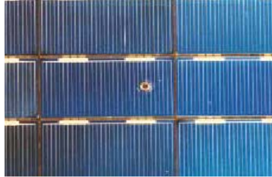
Figure 1. Photo of a Hubble Space Telescope (HST) solar cell that has been penetrated by space debris
